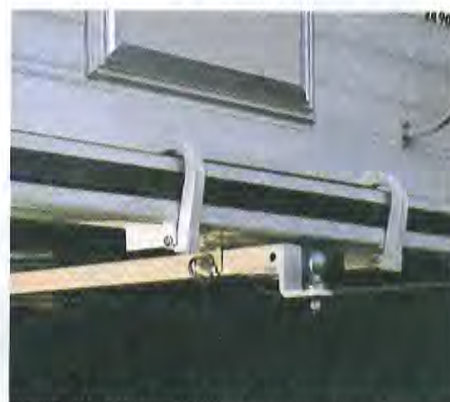
Class 1 tow bar. This bar attaches between the truck and camper bumpers.
