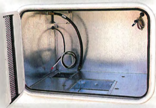
An optional pre-wired and fitted "generator-ready" compartment is available on larger Lance models and the Squire 8000.
