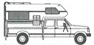
Standard cabover and crew cab pickup truck.
