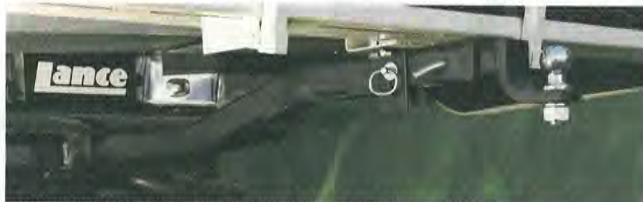
Truck-mounted receiver with extension tube, used with longer campers
